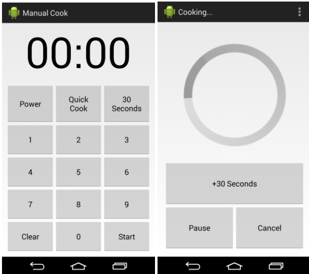
Fig 6. Allows the user to manually set cook time and power level like a standard microwave. During cooking the screen displays a circle to denote time.
